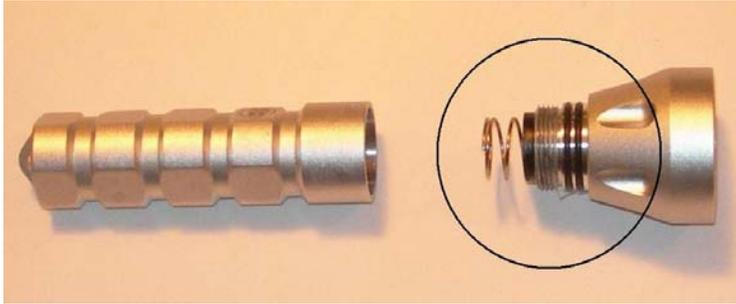
**Required Maintenance:** Apply an anti-seize compound to the threads of the flashlight head then apply silicone lubricant to the threads and O-Rings. Apply a minimal amount barely visible. Threads must be wiped off with a lint-free cloth and anti-seize compound must be applied at least every 2 months. More frequent maintenance may be required under harsh conditions or heavy use.
