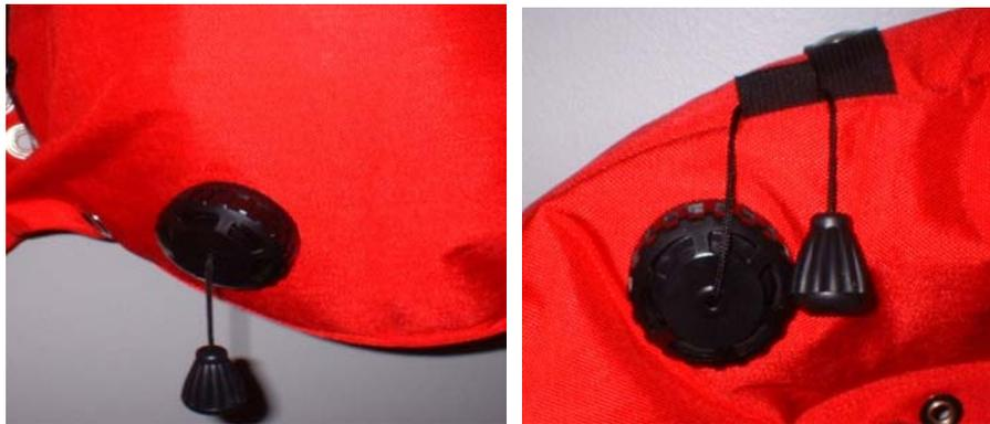
Pull dumps should be inspected regularly by fully inflating the BC to insure they vent properly. Also, be sure to thoroughly rinse them after each dive to prevent debris from becoming trapped in the seal causing air to leak from the BC.
