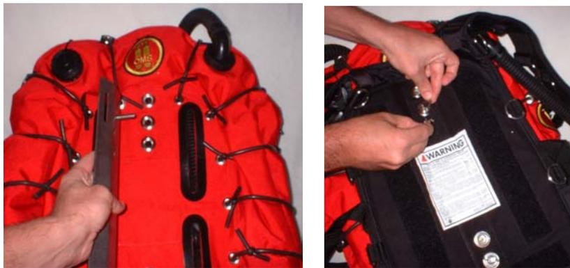
Install the flat washer first (against the backplate or harness) then the split lock washer. Thread the wingnuts onto the bolts and tighten securely by hand. Next install two nylon cam bands through the slots on the Single Tank Adaptor. Weave the webbing of the tank band through the cam buckle using the weave outlined on page 34. Remember, all nylon webbing stretches when wet so be sure to soak the nylon tank bands in water before tightening.
