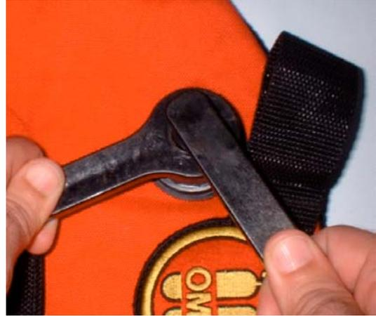
3. With the outer female fitting removed, the inner male fitting (Seal Ring part no. BCA 500) can be gently pushed back into the bladder exposing the double gasket.
